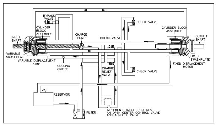
**BDU-21L/A Hydrostatic Flow Illustration**
