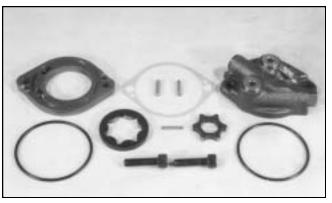
BDU-21L/A CW Charge Pump Components
