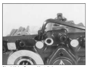
Check Valve Removal/Installation
