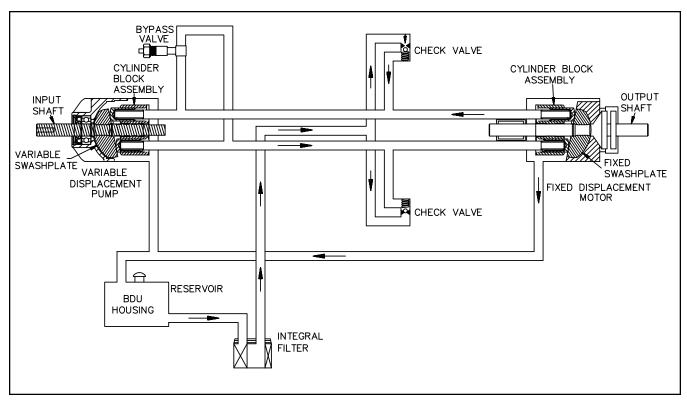
**BDU-10S Hydrostatic Flow Illustration**
