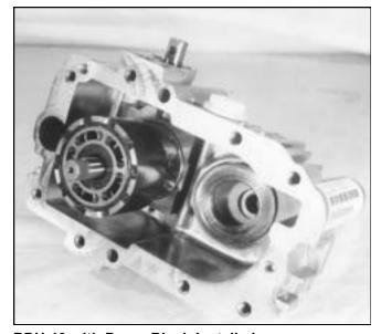
**BDU-10 with Pump Block Installed**
