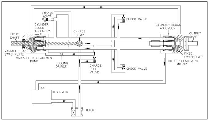
BDU-10L/21L Hydrostatic Flow Illustration
